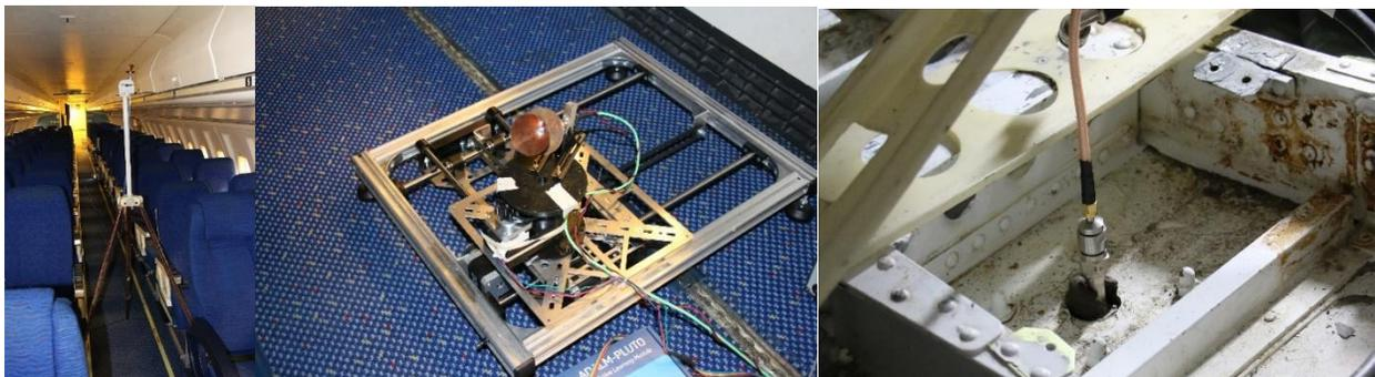
Figure 2: Photos of three different measurements: (1) transmitter used for measurement of aircraft shielding, (2) transmitter on positioner used for propagation measurements, and (3) receive equipment is attached to radio altimeter
