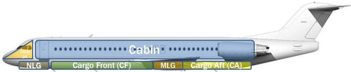
Figure 3: Compartmentation of the aircraft, where NLG and MLG stand for Nose/Main Landing Gear
